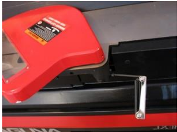
FIGURE 31: REMOVING GUARD FOR RABBETING
