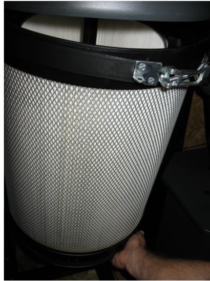
Figures 45-46: Disassembling canister for cleaning
