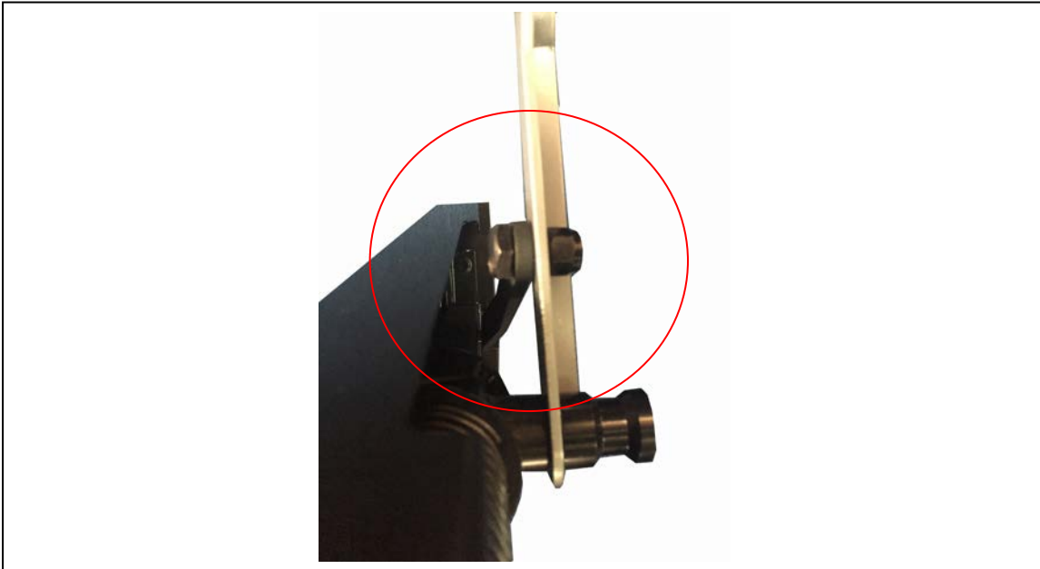
Figure 22: Securing support brace with foot pedal
