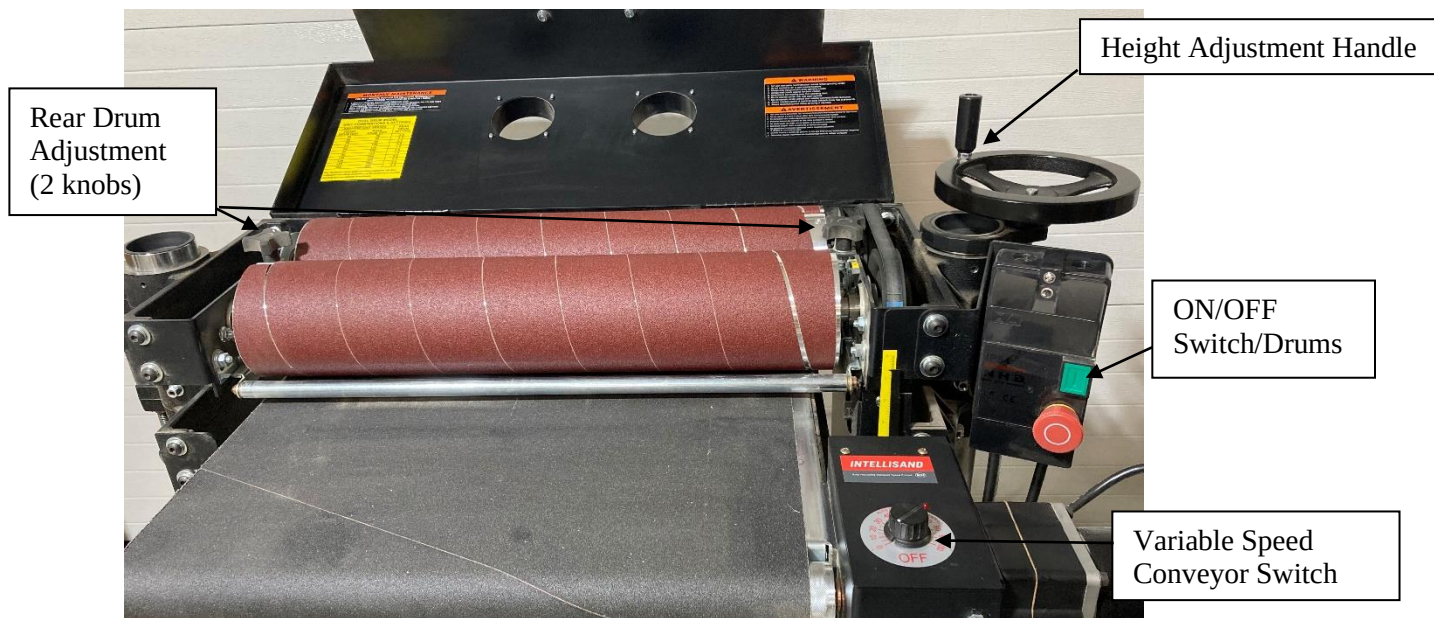
Fig. 11. SUPERMAX operating controls.
