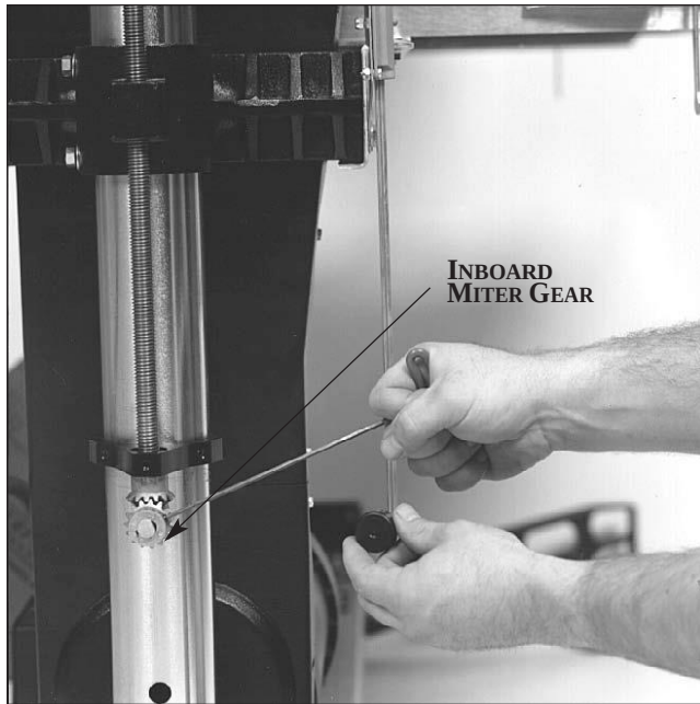
Fig. 6. Adjusting primary drum alignment.
