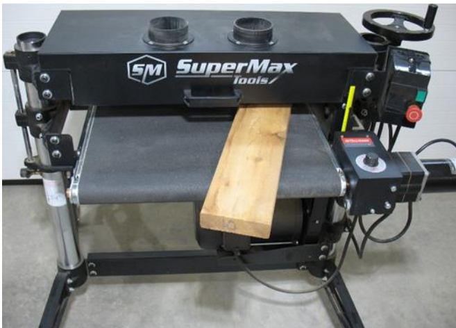
Fig. 15. Offset stock feeding angle.
