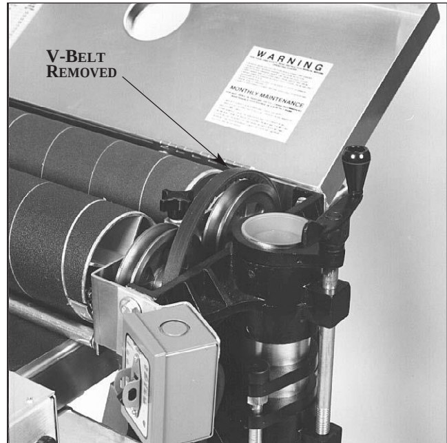
Fig. 30. Removing main motor V-belt drive.
