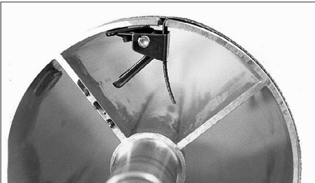
Fig. 10-d. Insert tapered end into outboard slot.
