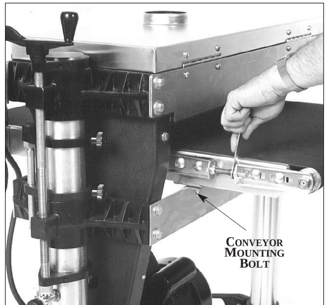
Fig. 28. Tensioning and tracking conveyor belt.
