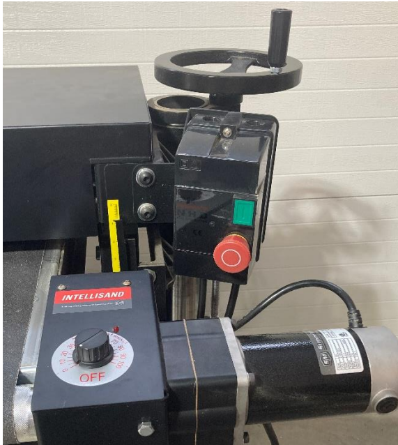
Fig. 31. Conveyor control box (Intellisand) and on/off switch.
